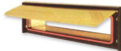
440 telescopic slots 2 3/4" x 10" (70 x 255) Seals front & back doors. Fits any door thickness. Polished brass, white or black finish.
